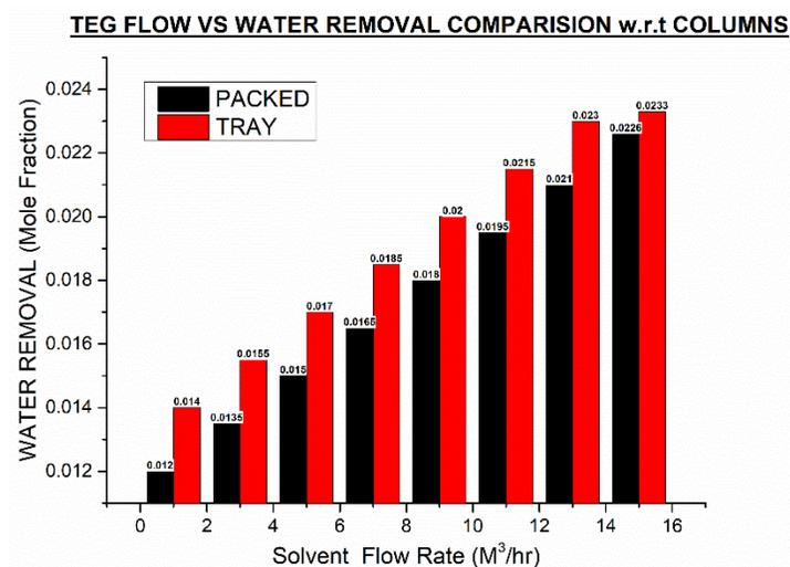
Fig. 07: Solvent flow vs water mole fraction for tray and packed column.
