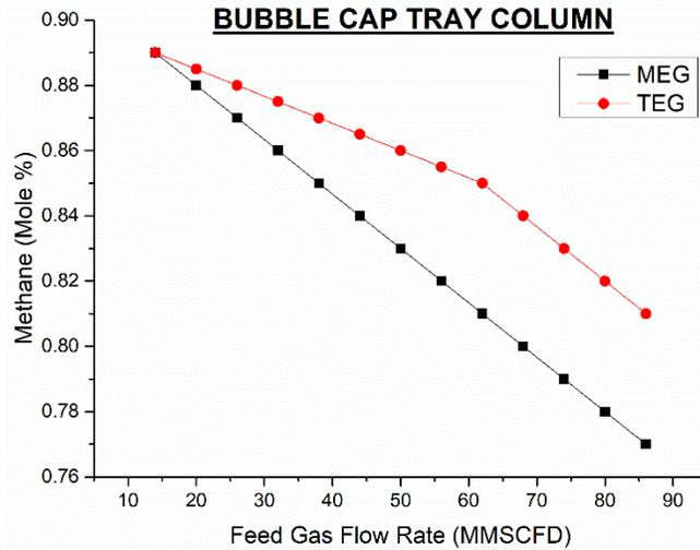
Fig. 08: Effect of feed gas flow on methane mole percent
