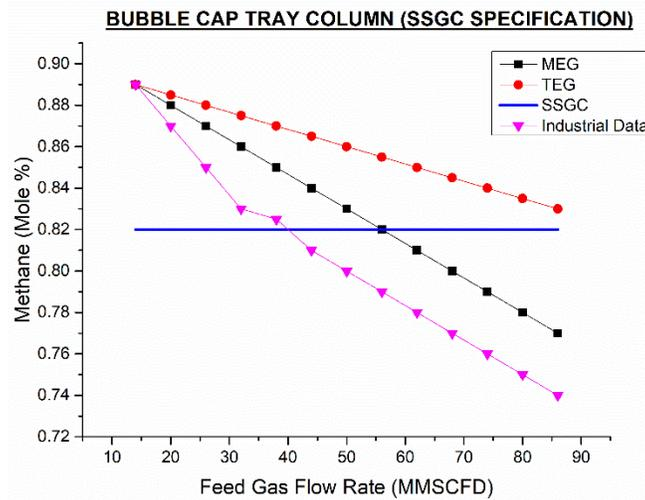
Fig. 06: Relation of gas flow rate at constant solvent flow with methane mole fraction.
