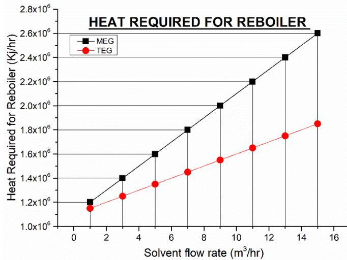
Fig. 09: Effect of solvent flow rate on reboiler heat requirement
