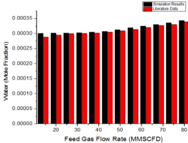
Fig. 05: comparison of simulation and literature results with feed gas flow rate and water vapor in dry gas
