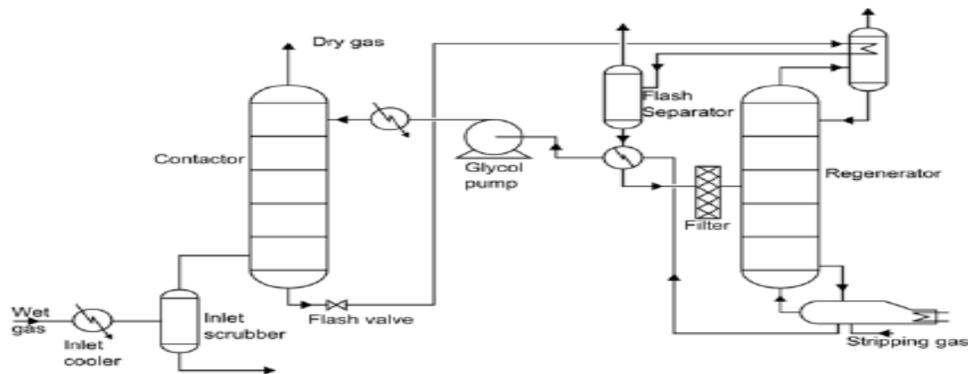
Fig. 01: Typical Gas dehydration process
